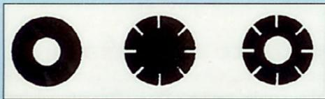
Figure 2. Common core diameters: notches and centre hole provide additional cooling capability
